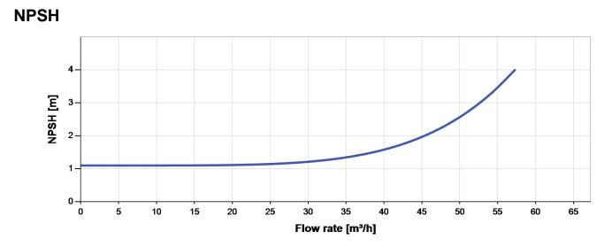
The NPSH (Net Positive Suction Head) is NOT the operating suction head. To calculate the operating suction head please refer to the installation manual.
